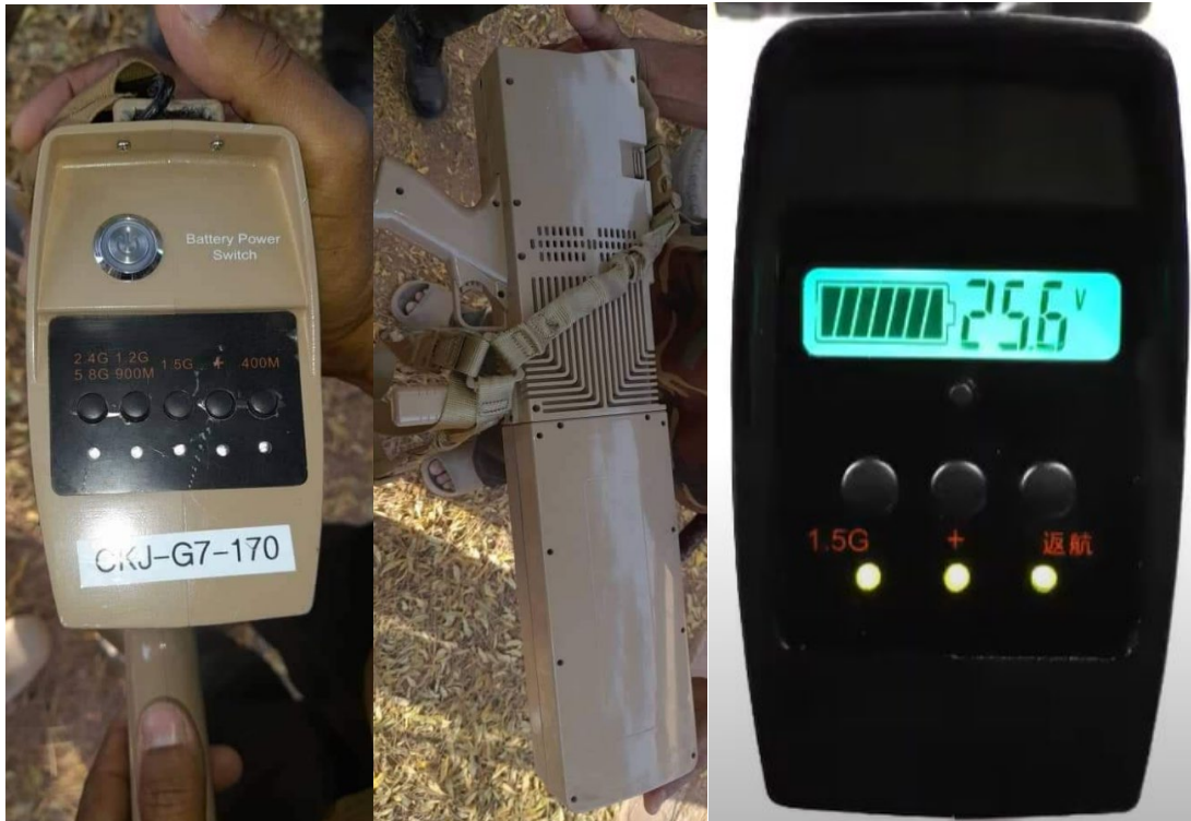
Left: Close-up of the drone jammers, with label marked CKJ-G7-170. 132 Right: control panel of CKJ jammers, as sold online. 133
