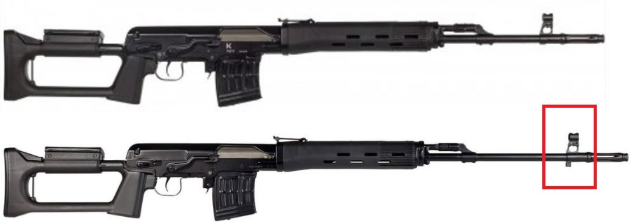
Above: A Tigr vers 1 (mod 2). 92 Below: a modern SVD, with the bayonet lug highlighted. 93
