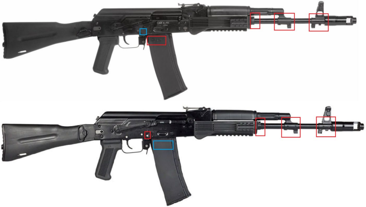
Top image: Saiga-MK 223 Rem. 102 Below: AK-101 103 The Saiga MK has its gas block and front sight pinned to the barrel, as opposed to the AK-101, where they are press-fitted. Additionally, the Saiga-MK lacks an additional rivet immediately above the magazine release catch, and are marked "223 rem" on the magazine.
